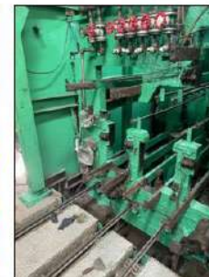
Entry looper bracket for arm swing and column structure repair
