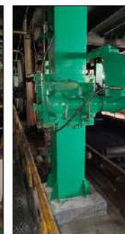
Entry looper bracket for arm swing and column structure repair
