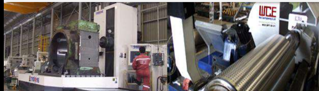
CNC Boring Machine
