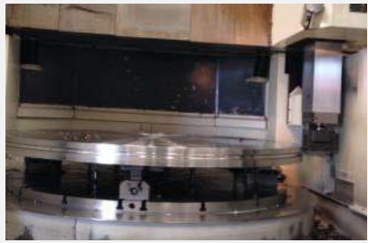
Jig for Seal ring housing Row#4
