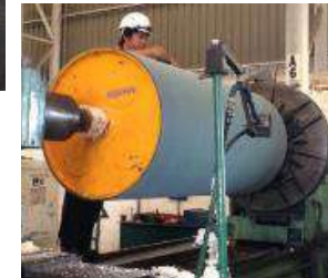
Wheel for Chock 1 CW (Material: SCM440 Induction 45-50 HRC)
